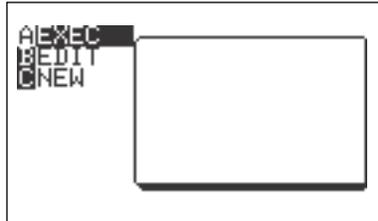
2. Press **C** (**NEW**) and **ENTER** to open a new program. The calculator is now locked in ALPHA mode and is prepared to accept a name for the new program. Enter the program name.
