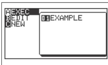
3. If you receive an error statement, press **◀** **▶** to go to the line within the program in which the error occurs. Compare your line with the correct one above to find the error. Correct the error using the editing features of the calculator and press **ENTER** to save the correction. Press **2ndF** **QUIT** and try to execute the program again.
